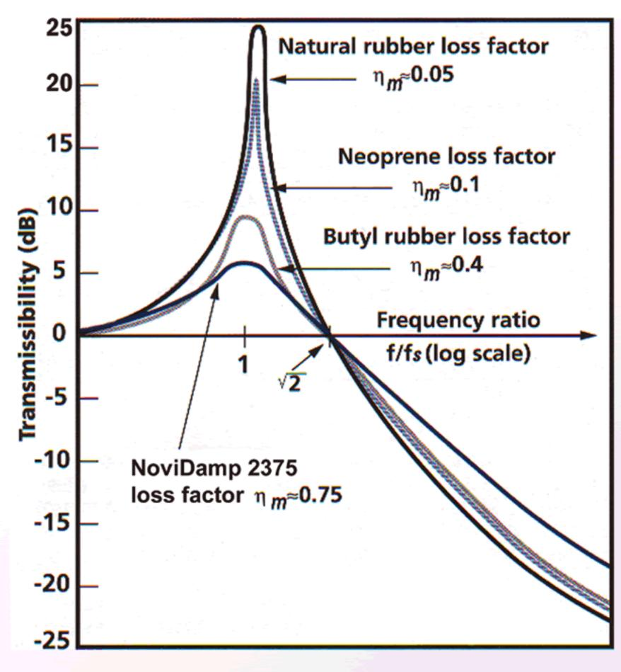
Uncontrolled response of rubber and other poorly damped elastomeric isolators can mean audible noise in typical operation environments. Novidamp 2375 minimizes these effects.
